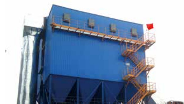
Bag filter for slag grinding system of Zhangjiakou Liaoyuan Cement Co. Ltd.(0.3 Mt/a)
