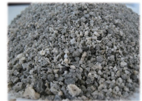
高炉矿渣 Granulated blast furnace slag
