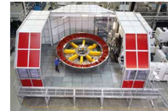
GERMANY NILES GRINDING MACHINE ZP80 8-meter in China The largest precision gear grinding machine in the world, max. gear diameter 8 M, also it is the only set in the world.
