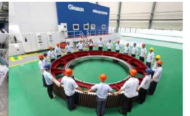
GERMANY GLEASON-PFAUTER NC-HOBBING 10-meter in China High Efficiency and Precision Hobbing Machine, Max. machining diameter 10 meters
