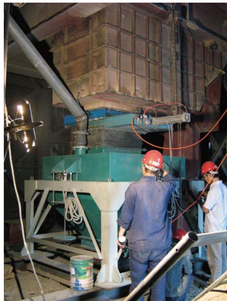
图3 TSMS3000熟料计量秤现场应用图 Figure 3 TSMS3000 Clinker Weigh Scale under commissioning
