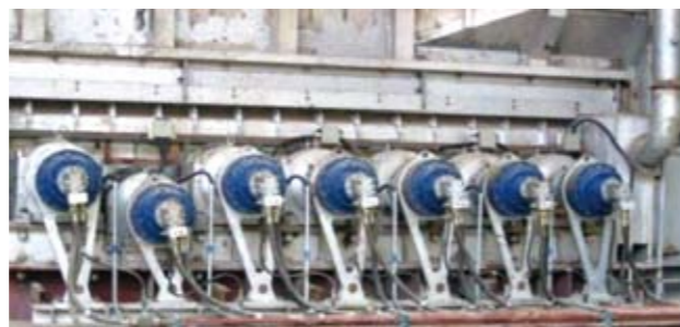
自主研发的带中间辊破的新型高效第四代篦式冷却机 Self-developed New Type High Efficiency Grate Cooler with Roller Crusher in Middle
