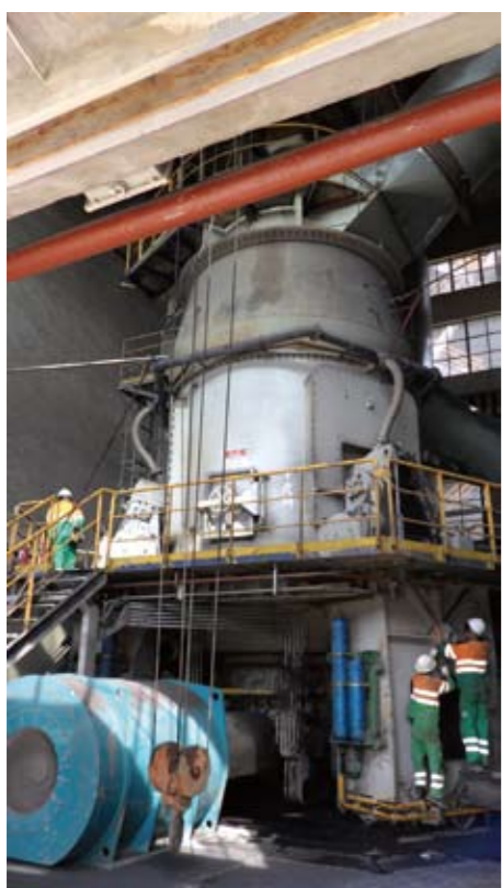
拉法基三岔TRMC31.3磨机的外形 Sketch of TRMC31.3 at Lafarge Sancha project
