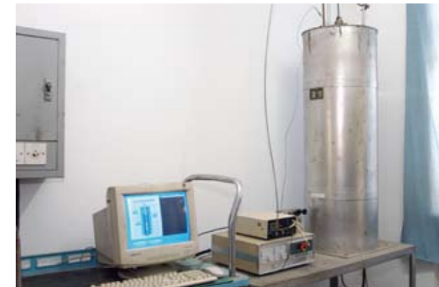
煤燃尽试验装置 Coal Burnout Test Instrument
