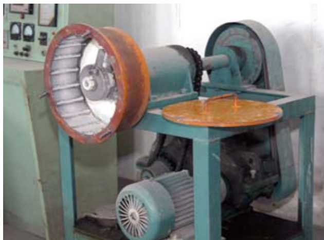
磨蚀机 Abrasiveness Test Mill
