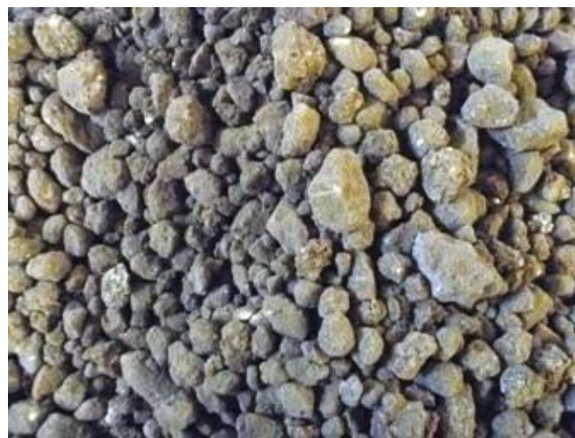
硫铝酸盐水泥熟料的外观 Clinker of Sulphoaluminate Cement
