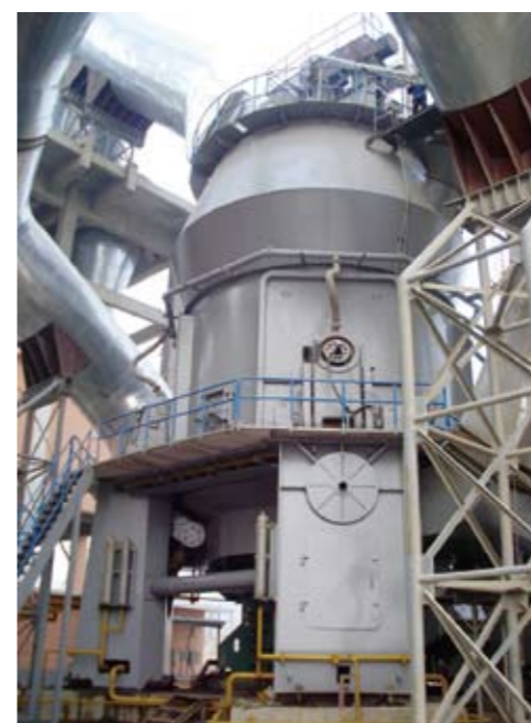
●河北燕赵TRM53.4磨机的外形 Outline of TRM53.4 Of Hebei Yanzhao cement co., Ltd
