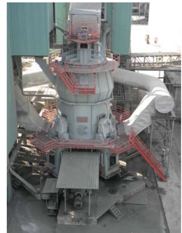
● 幸福水泥TRMK4541磨机的外形 Outline of TRMK4541 of vietnam phuc son cement co., Ltd owned by Taiwan lucky cement group
