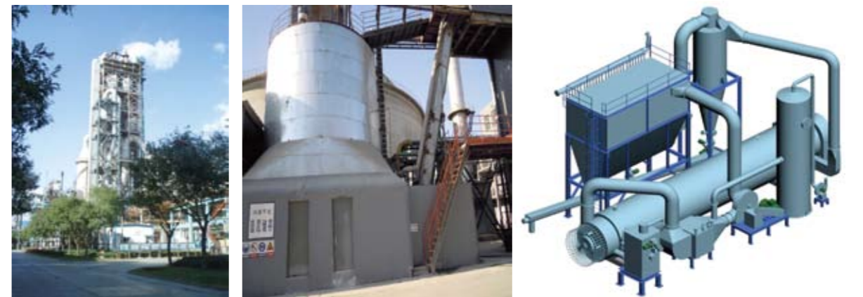
协同处置污泥生产线 Sludge disposal production line 湿污泥储存输送系统 Wet sludge storage and delivery system 污泥干化系统模拟图 Simulation diagram of Sludge drying system
