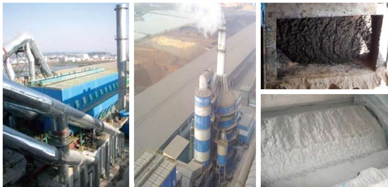
污泥干化及分离收集 Sludge drying and separating collection 干化尾气除臭 drying waste gas for deodorization 干化前后污泥形态 sludge before and after drying
